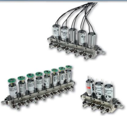
The standard solenoid valve block of 1.4305 is used for stream switching up to 10 different streams. It has rapid switching solenoid valves, which have a very long life time – tested over 500 million switching operations. Due to the small design the solenoid valve block can be installed in an 19"-rack directly behind the analyzer.
